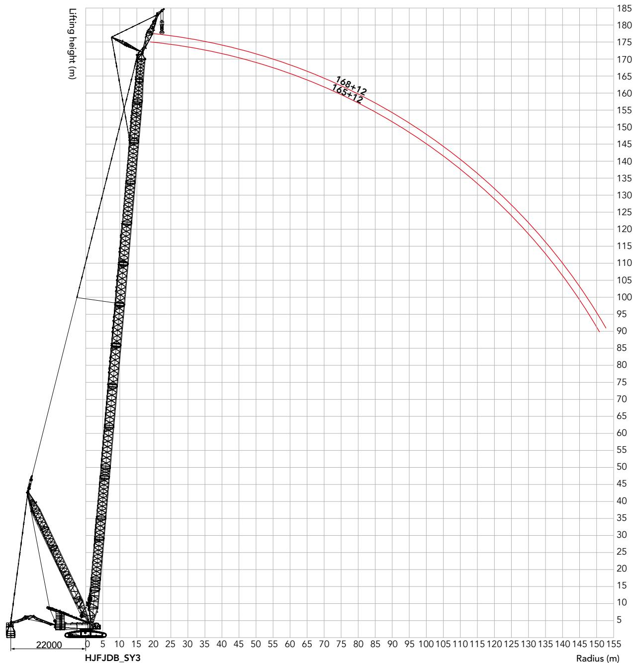
**Load Chart of HJFJDB\_SY3 Configuration****SCC8000A Crawler Crane - HJFJDB\_SY3 1/3**
