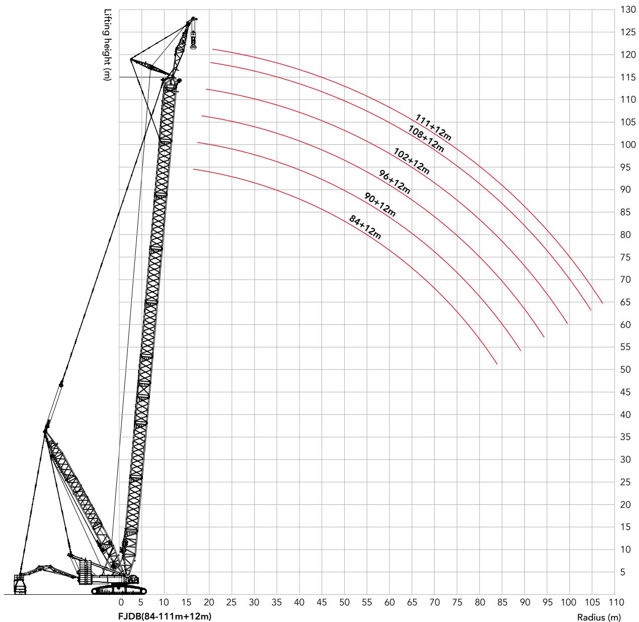
**Load Chart of FJDB Configuration****SCC8000A Crawler Crane - FJDB 1/3**
