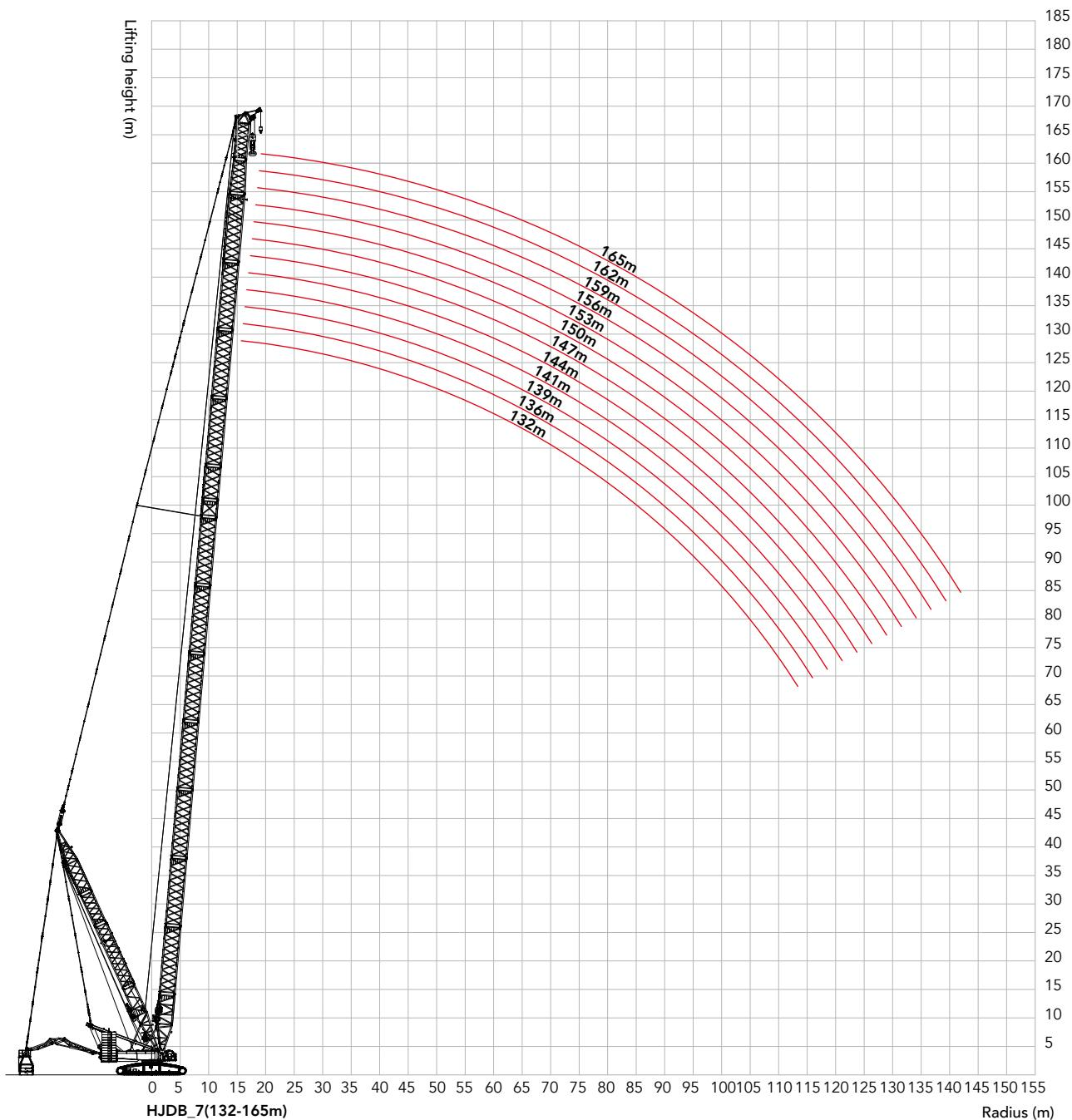
**Load Chart of HJDB\_7 Configuration****SCC8000A Crawler Crane - HJDB\_7**
