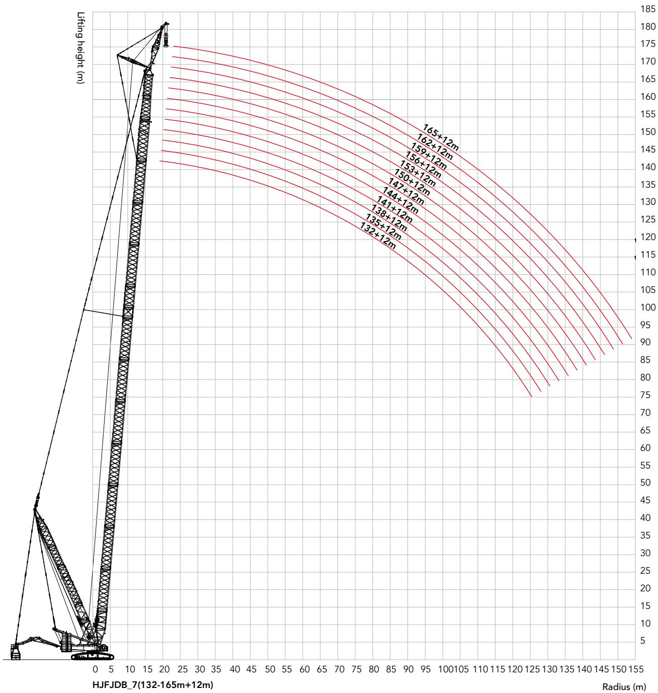
**Load Chart of HJFJDB\_7 Configuration****SCC8000A Crawler Crane - HJFJDB\_7 1/3**
