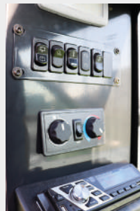
Air conditioning, heating, radio controls
